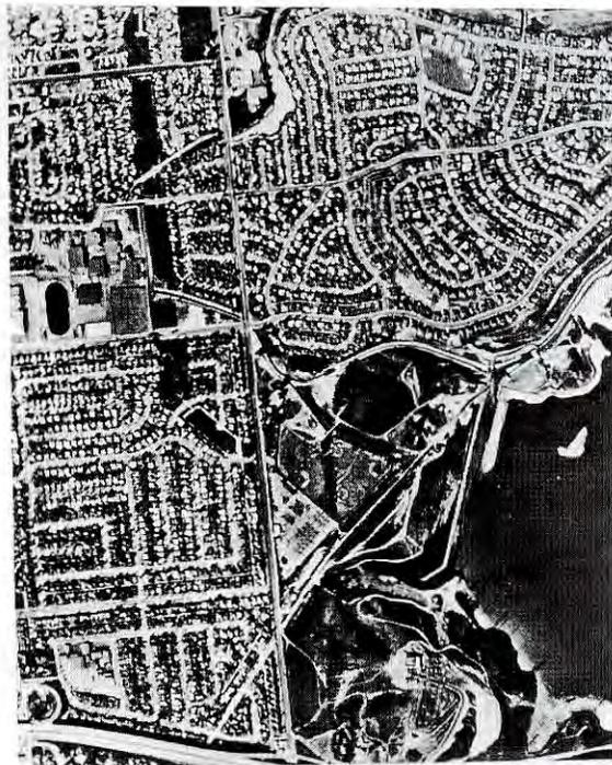
FIGURE 43. Damaged Lower San Fernando Dam one day after the February 9, 1971 San Fernando California earthquake (M<sub>s</sub> = 6.4) and its relation to the densely built-up area downstream. The school at the left edge of the photograph is a school. (National Aeronautics and Space Administration, photograph from Rash, M., Holguin, A., and Vernon, S., *Potential Role of Remote Sensing in Earthquake Management*, School of Public Health, University of Texas, Houston, no date, 49A. WJ)
