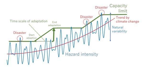
Schematic view of hazard and acceptance level including adaptation (blue: hazard intensity (e.g., water level), green: limit of capacity (e.g., dike height), red: climate change trend)
